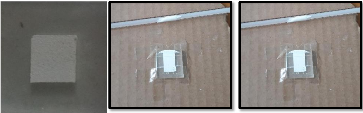
Fig. 2. Paste depositions with the doctor blade method.
